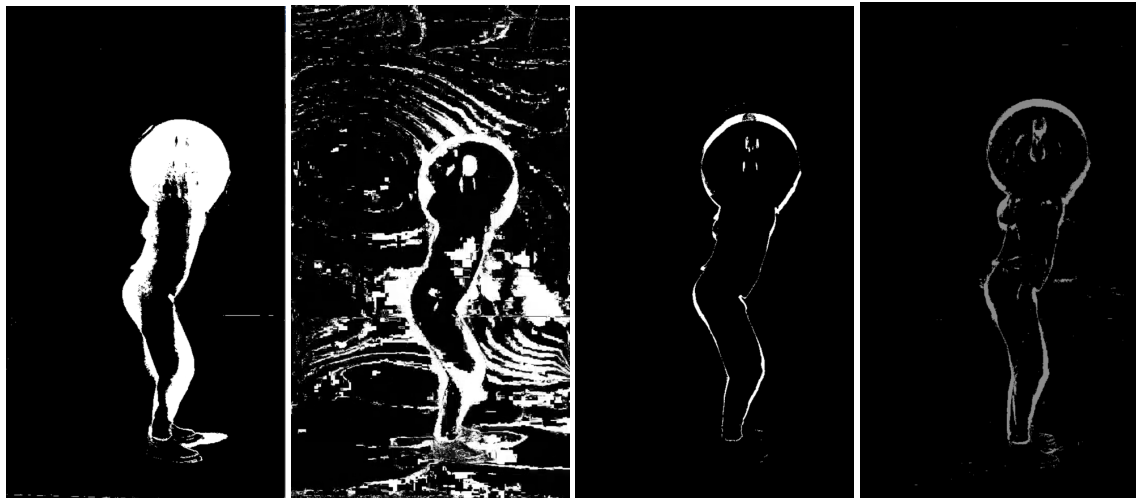
Figure 6.1 Background subtractor processed image (a)CNT (b) GMG (c) MOG (d) MOG2
